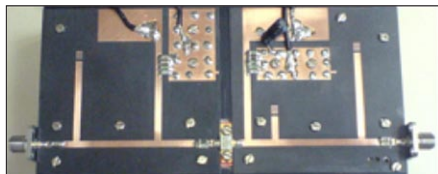
Fig.2: Highly efficient, narrowband Class-J PA.
